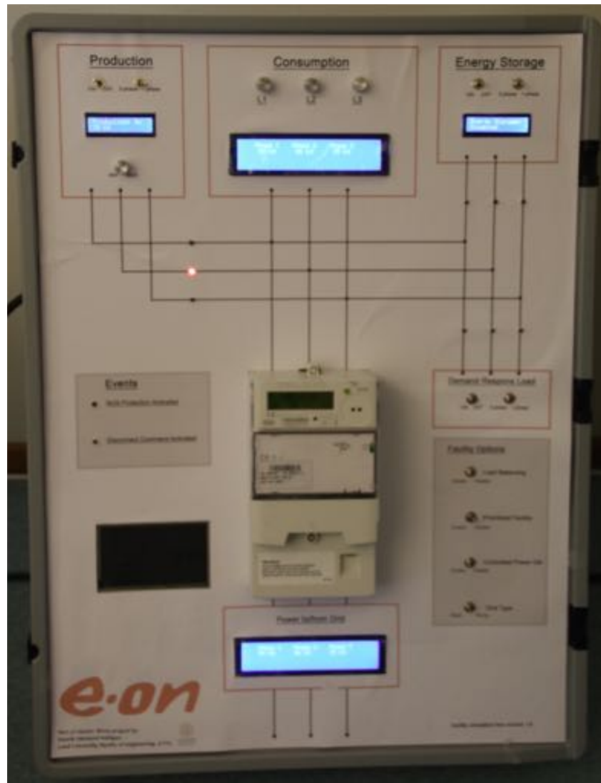
Figure 20, Facility platform box
