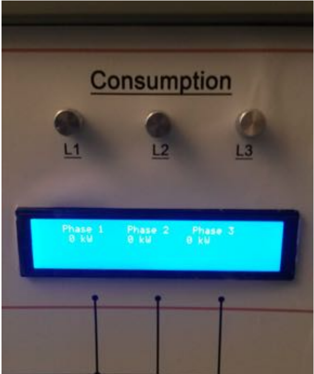
Figure 43, Consumption to zero to indicate that the meter has switched off.
