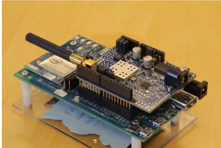
Figure 6, Intel Edison with Connode radio module mounted
