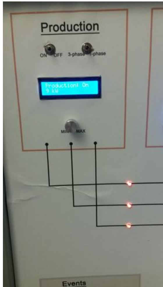
Figure 33, Production section of facility platform. State = On. 9 kW three-phase
