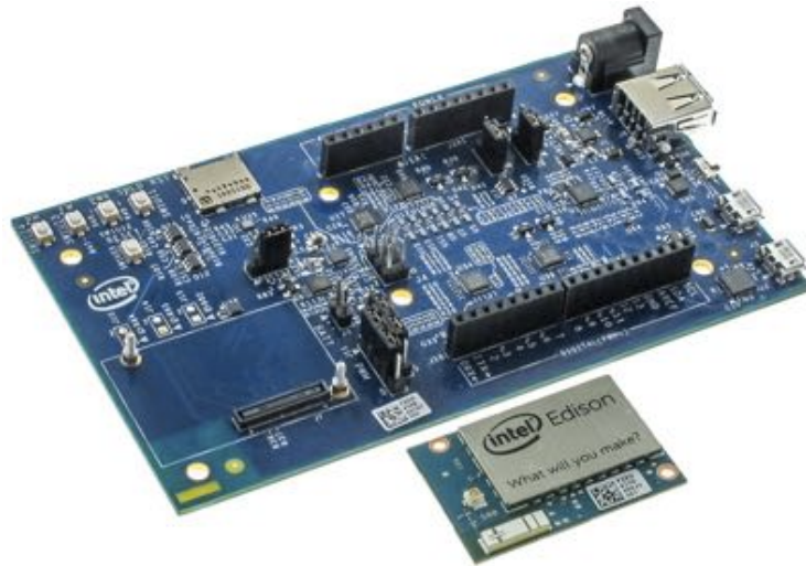
Figure 7, Intel Edison SOC (35 x 25 mm) and the larger Arduino Breakout board, (125 x 70 mm)
